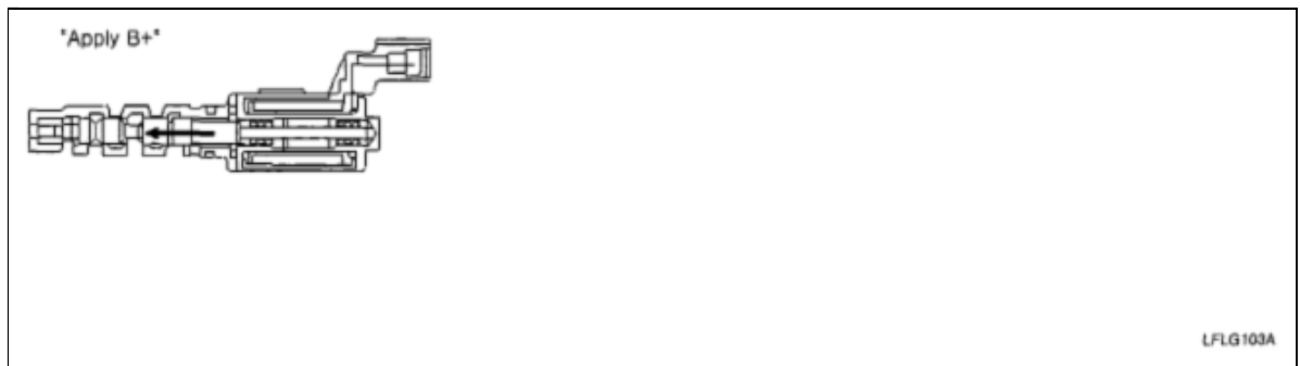
Fig 5: Checking OCV Operation
